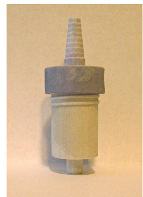
Figure 14. Prototype 3 is a modification of prototype 2 and was made of proprietary plaster powder and cyanoacrylate glue, with a steel ball and rubber stopper inserted. A screw-on cap was included for ease of fabrication. The Christmas tree on top of the cap allows for easy connection to the vacuum and the cylindrical attachment on the bottom can attach to the trap. Dimensions can be found in Appendix C.
