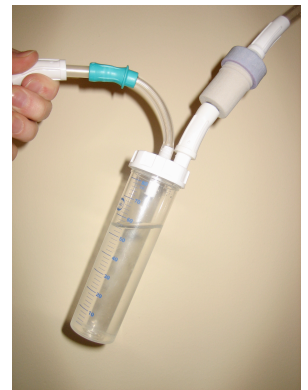
Figure 17. Final prototype connected to specimen trap representing connection to bronchoscope and vacuum.
