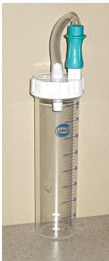
Figure 4. The tubing on specimen trap that connects to the scope can be attached to the vacuum connection to enclose the system.
