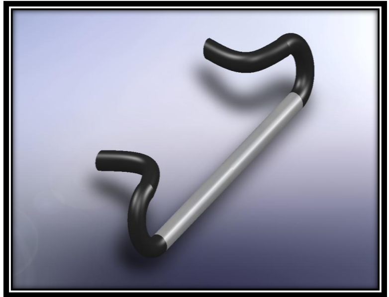
Figure 7 - U-Shape design. The light colored rod represents stainless steel. Black colored components represent flexible rubber joints.
