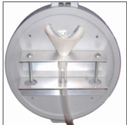
Figure 16: Loading Mechanism and L-Brackets
