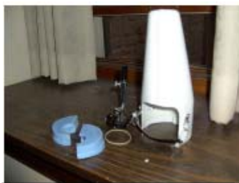
Figure 3 The silicone rubber insert, microdrive unit, watchstrap and outer shell from the prototype.
