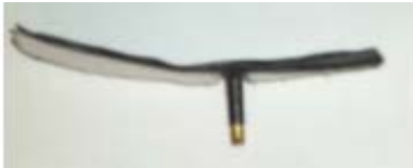
Figure 5 The inflatable air bladder cushions the monkeys' skulls and keeps the helmet securely on their heads.
