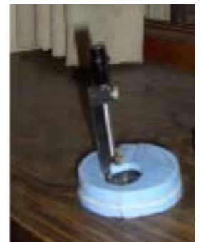
Figure 4 The silicone rubber fits tightly around the microdrive unit.
