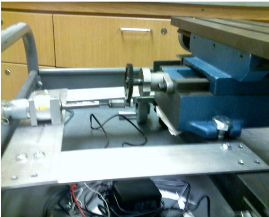
Figure 4: The motor attachment to the rectangular base.
