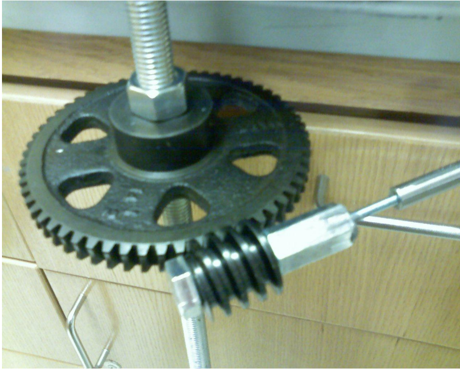
Figure 3: Rotation gear mechanism. The metal shaft is bolted to the table so that when the gear is spun, the table rotates.
