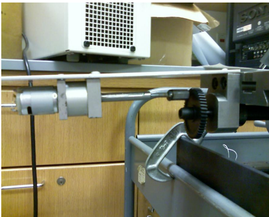
Figure 2: Two gear system for moving the device in the other horizontal direction. No gear is pictured two to it break during tapping.
