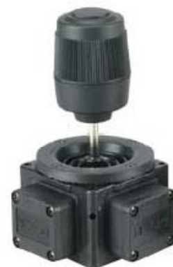
Figure 11: Joystick that will control all three degrees of motion.
