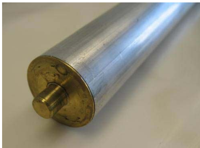
Figure 7: The integrated hinge design would have a pin and hole assembly allowing for easier fabrication. However, this would increase the amount of friction and reduce the efficiency of the transport.
