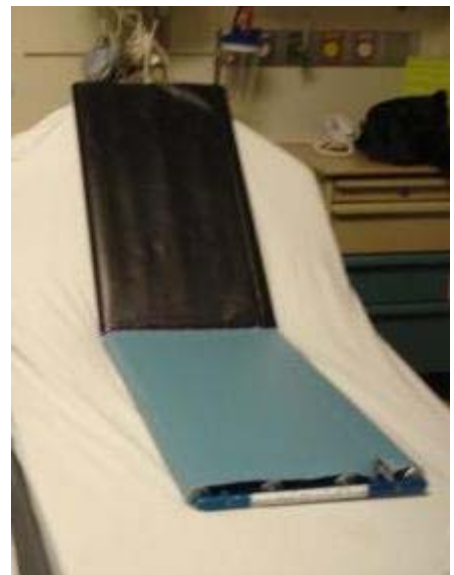
Figure 6: The two existing boards design would simply link two boards with a hinge in the middle. The final product would look very similar to this figure.
