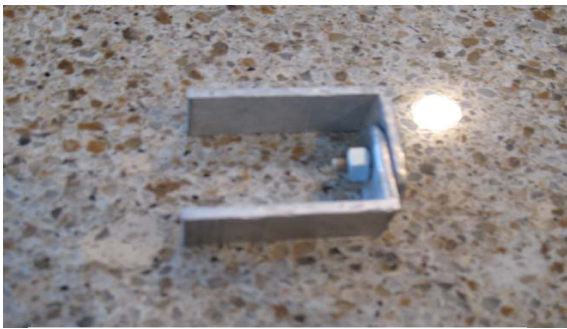
Figure 6: L-Shaped Hinge The L-shaped hinge is small, lightweight, and reliable.
