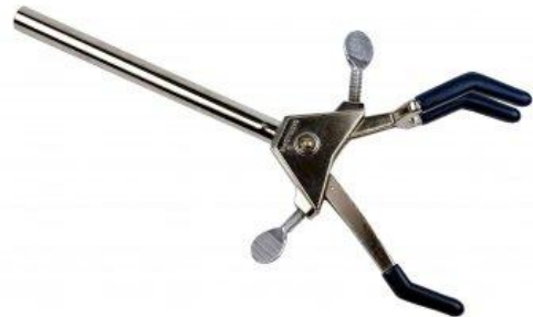
Figure 8. A three prong clamp that could be used to hold the probes in position. The two screws are used to tighten the clamp when it is in the correct position.
