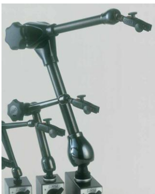
Figure 6 - Several Articulated Arm models. One knob at the corner joint tightens all three joints, allowing size degrees of freedom with one adjustment. From Noga Engineering.
