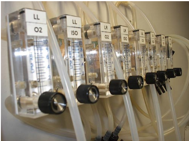
Figure 1. Isoflurane delivery system. Knobs are manually adjusted by an operator to mix appropriate amounts of isoflurane and oxygen in administering the proper concentration of anesthesia.
