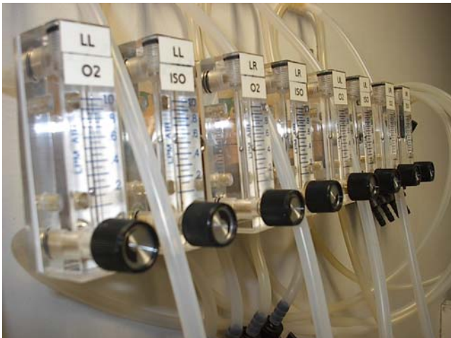
Figure 6. Isoflurane delivery system. Knobs are manually adjusted by an operator to mix appropriate amounts of isoflurane and oxygen in administering the proper concentration of anesthesia.
