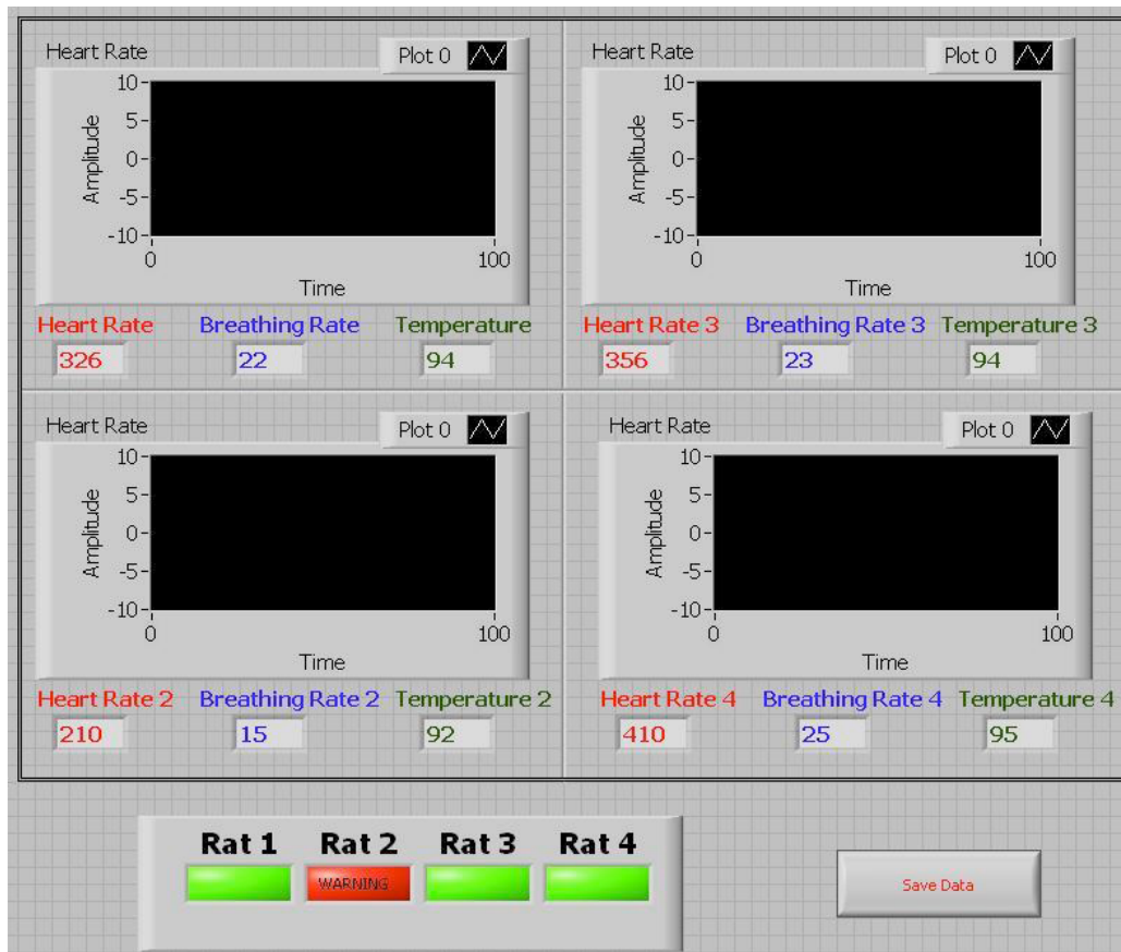
Figure 12. Design of user interface. Graphs are used to display the plethysmographic waveforms of each rat. Heart rate, breathing rate, and temperature will be shown numerically underneath. Warning lights will also be placed underneath alerting the user if a rat has fallen into dangerous conditions.
