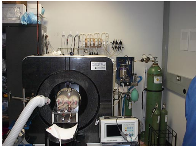
Figure 5. This picture shows the current set up of our client's PET imaging machine. Four rats are placed into the machine, two rats stacked on top of the other two. The pulse oximeter our client is currently using to monitor heart rate and SpO 2 levels is to the right of the PET machine.
