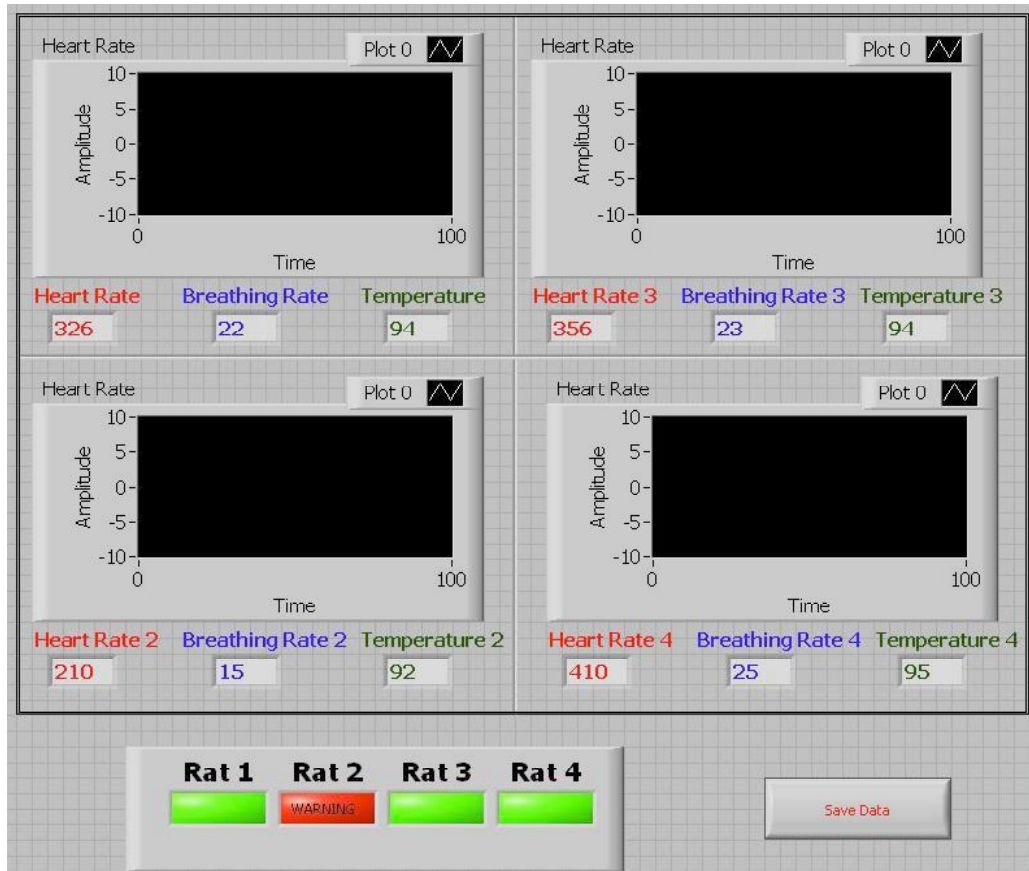
Figure 17. Design of user interface. Graphs are used to display the plethysmographic waveforms of each rat. Heart rate, breathing rate, and temperature will be shown numerically underneath. Warning lights will also be placed underneath alerting the user if a rat has fallen into dangerous conditions.
