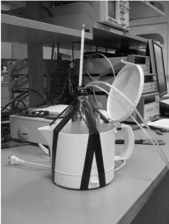
Fig. 4. The experimental set-up of the temperature test. The glass container was taped to the to the waterbath to keep it from floating.
