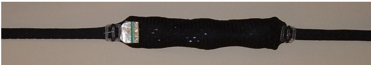
Figure 9 Extended strap without alarm circuit.
