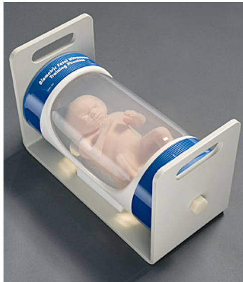
Figure 2- Fetal biometrics phantom manufactured by CIRS Inc.
