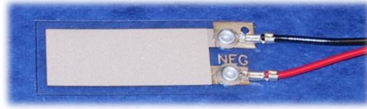
Fig. B-1. Piezoelectric film used to construct sensors for training model. [2]
