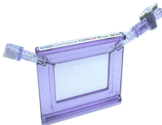
Figure 2: The CLINICell cassette provides the most competition to our design proposal in that it allows perfusion culture with adherent cells. However, the geometry of the cassette is not optimized for flow distribution, the plates are too thin, allowing oxygen permeability, and the cassette size is too small for our purposes
