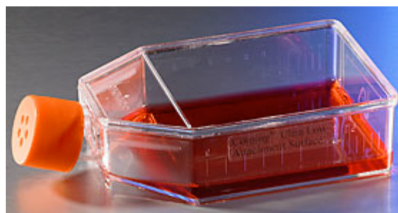
Figure 1: Static cell culture flasks sold by Corning (Product #3814) are frequently used to grow cells. The cells are attached to the bottom and are bathed in liquid media as shown.
