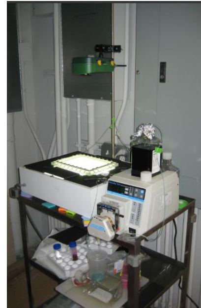
Figure 13. Example of dye experiment setup. Cassette was placed on illuminated surface and secured underneath a time lapse camera. A pulsatile pump supplied a flow rate of 3 fluid exchanges per day.
