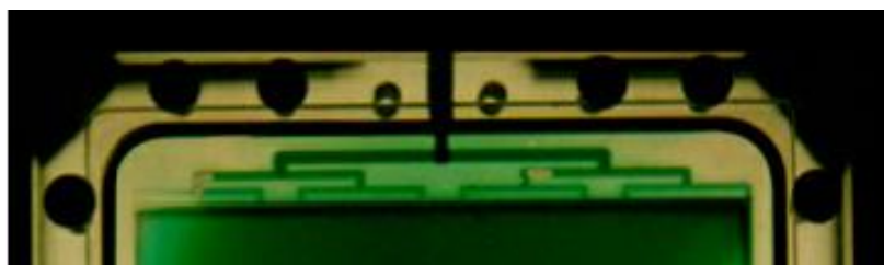
Figure 18. Bubbles lodge in the network of the balanced runner design, can affect flow, and are difficult to remove. Note lack of fluid delivery to section blocked by bubble.
