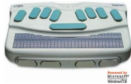
Figure 6 – HumanWare's Braille Note is used by the visually impaired to read computer screens
