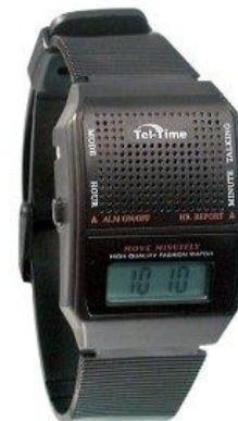
Figure 2 - The Audible Watch announces the time to the user when prompted
