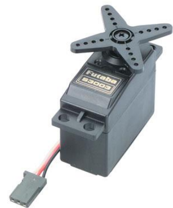
Figure 9 - Servos will be used to rotate the disks containing the Braille dots
