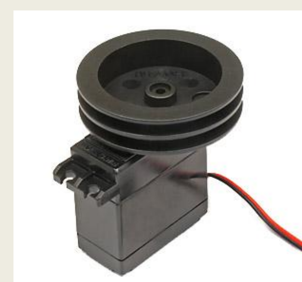
Figure 5: High torque full turn GW servos are used to rotate the Braille disks
