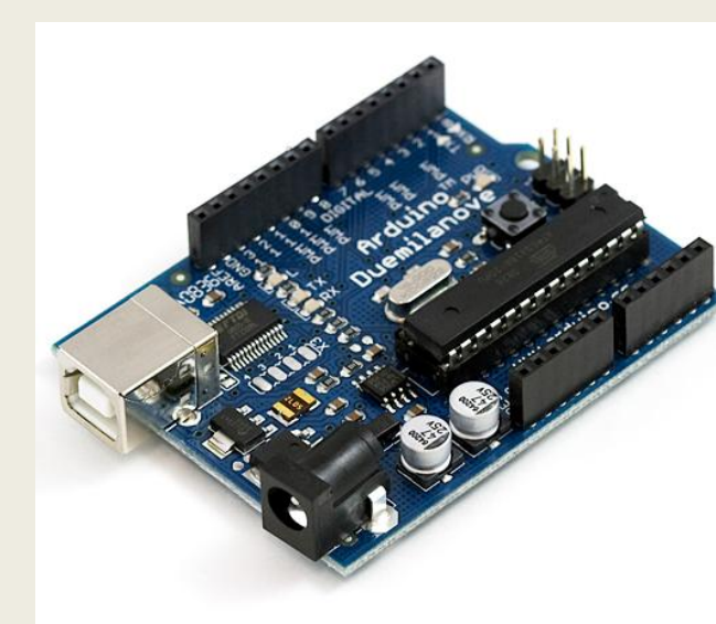
Figure 3: An Arduino Duemilanove microcontroller programs the watch
