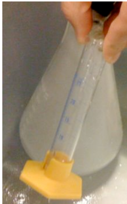
Figure 19 An Erlenmeyer flask with an outlet port was used to collect rainout of the albuterol mist into a graduated cylinder.
