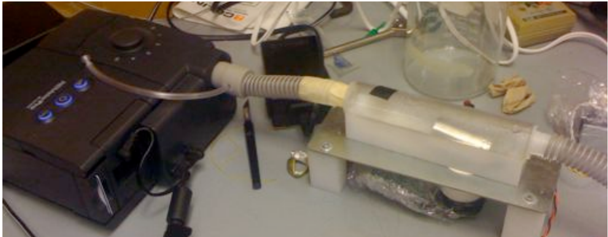
Figure 18 Orientation of CPAP nebulization device during testing of the delivery of aerosol to the CPAP mask.
