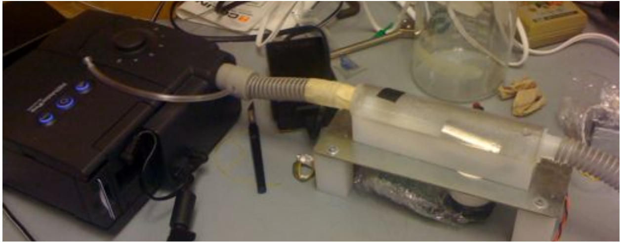
Figure 9 Orientation of CPAP nebulization device during testing of the delivery of aerosol to the CPAP mask.
