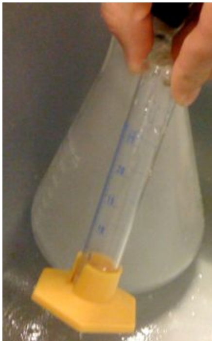
Figure 10 An Erlenmeyer flask with an outlet port was used to collect rainout of the albuterol mist into a graduated cylinder.
