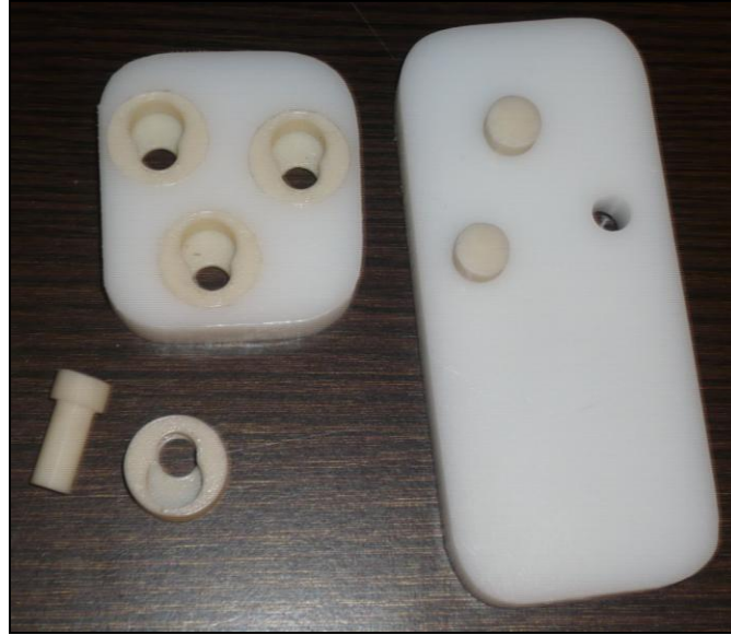
Figure 14: This is an image of the initial enlarged prototype of the vertical track design. Three vertical slots have been implanted in the smaller piece, which represents the ear. The larger piece represents the skull and has three enlarged abutments.
