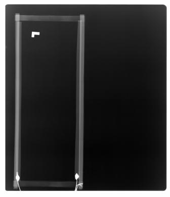
• Image with no phantom. Image analysis software calculated less than 3.9% attenuation. (Peppler, 2009)
