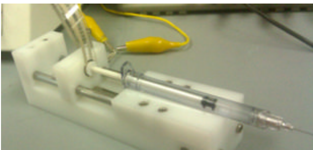
Figure 11: Block design shown with FlexiForce sensor attached and syringe placed in position with 25 gauge needle.
