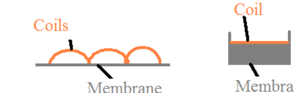
Hand wound coils (left) vs. photolithography coils (right)
