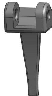
Figure 3: The metacarpal component is made of CoCr.
