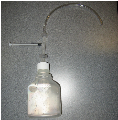
Figure 9: Prototype of final design (without BB) attached to a sample bottle with the same
