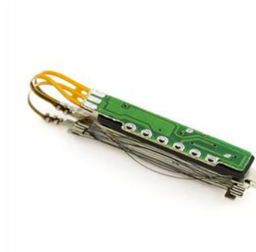
Figure 9: Shape memory alloy actuator. http://www.sparkfun.com
