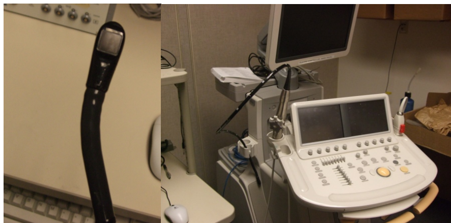
Figure 2: Philips X7-2T ultrasound probe and accompanying ultrasound machine. Image taken February 1 st , 2010.
