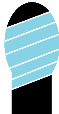
Figure 3: Drawing of liquid tubing design. The tubing will be wrapped around the tip and saline will flow through the tubing.
