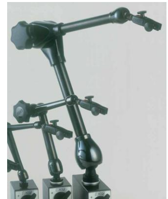
Figure 4 - Several Articulated Arm models. One knob at the corner joint tightens all three joints, allowing size degrees of freedom with one adjustment. From Noga Engineering.
