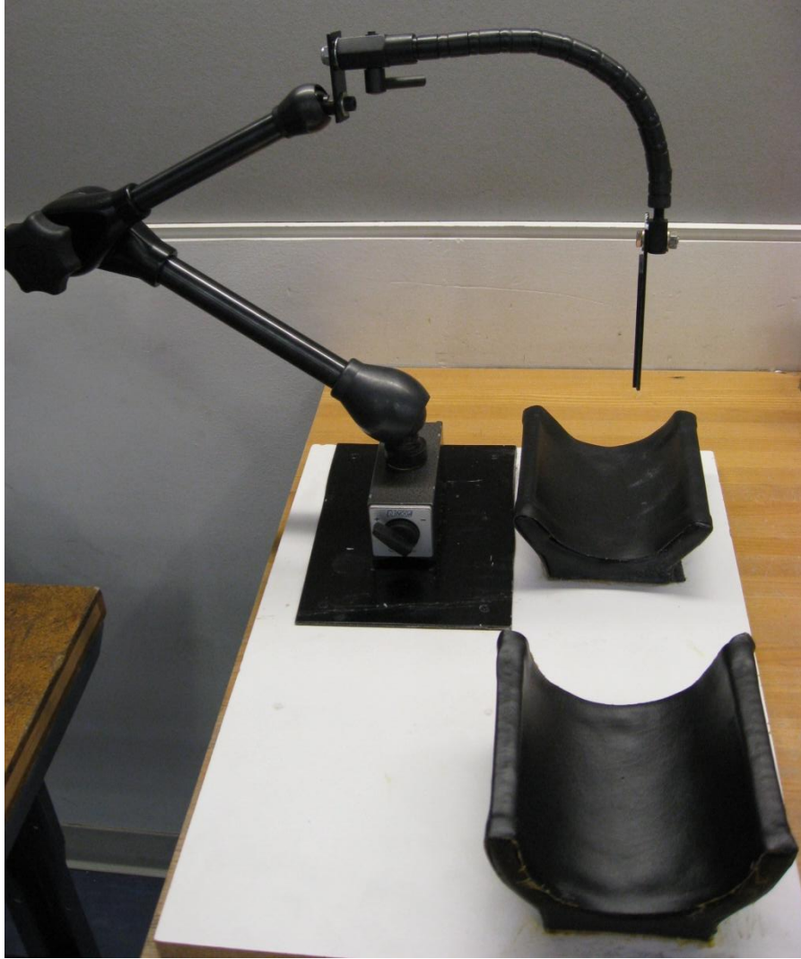
Figure 10 – Final design combining the hybrid positioning mechanism and the Velcro strap clamping mechanism.
