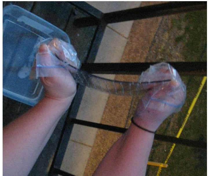
Figure 11 Material Durability Testing - bending the polycarbonate to assess its rigidity
