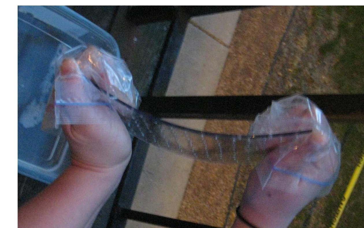
Clamp degradation testing polycarbonate. Increased rigidity after soaking in formalin for 2 hour time period
