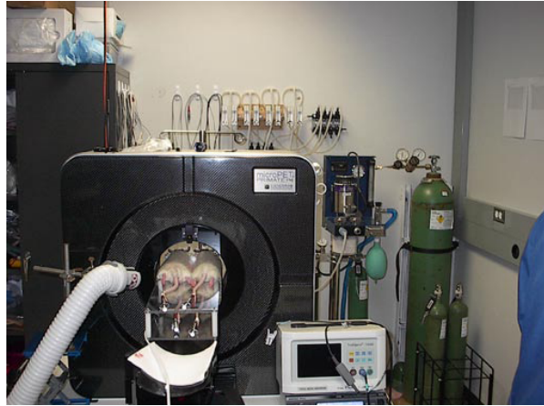
Figure 1: This picture shows four rats in the PET scanner at the client's laboratory. The rats are oriented in a two by two square [1].
