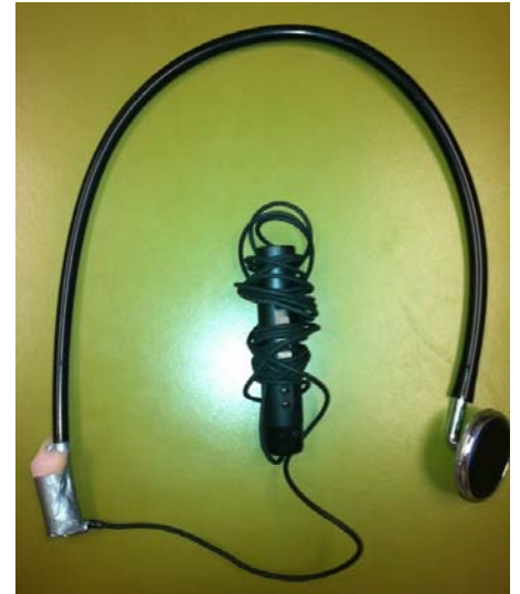
Figure 3: Recording Apparatus used to obtain heart and breath sounds samples.
