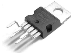
Figure 20: TDA2003 Power Amplifier used to power the external speakers
