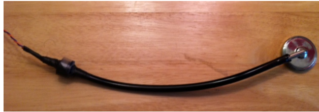
Figure 15: Stethoscope bell with microphone coupling mated with rubber tube
