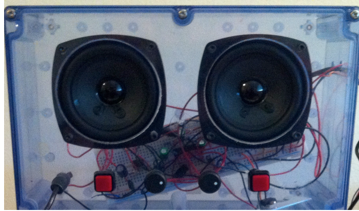
Figure 18: Front view of control panel. From left to right: headphone jack, Speaker power switch, headphone volume, speaker volume, On/Off.
