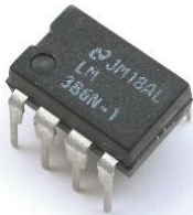
Figure 19: LM386N operational amplifier to power the headphones
