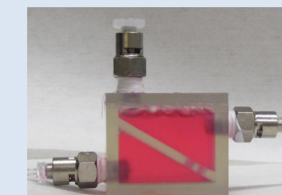
Figure 6: Exterior bubble trap
