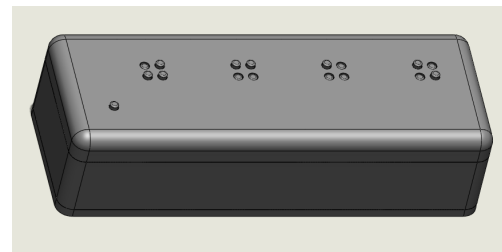
Figure 5: Final Braille Watch assembly displaying the time 03:15 PM
