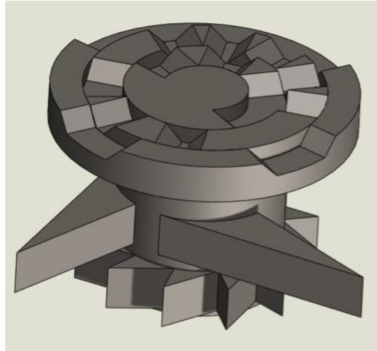
Figure 13: A disk with different combinations of raised and lowered segments can display a desired range of numbers
