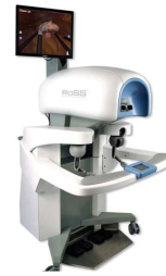
Figure 3. RoSS virtual surgical simulator (Simulated Surgical Systems).
