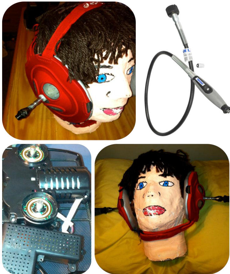
Figure 5. Final prototype (Clockwise from top left): headgear with Dremel attachments; Dremel flexible shaft; device with Dremel shafts attached; motor and electrical controller
