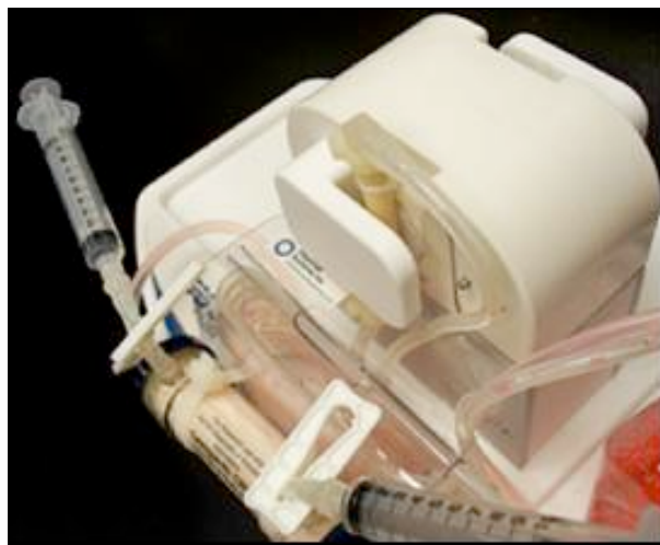
Figure 12: Duet pump used with hollow fiber bioreactors. This positive pressure displacement pump squeezes the inserted tubing, while using integrated one-way check valves to determine the direction of flow [6] .
