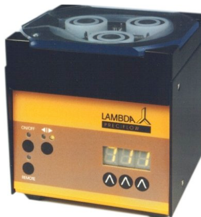
Figure 11: Peristaltic pump with glass bead bearings to compress the tubing and direct flow by the same means as a standard peristaltic pump, but with a reduced pulsation effect [14] .
