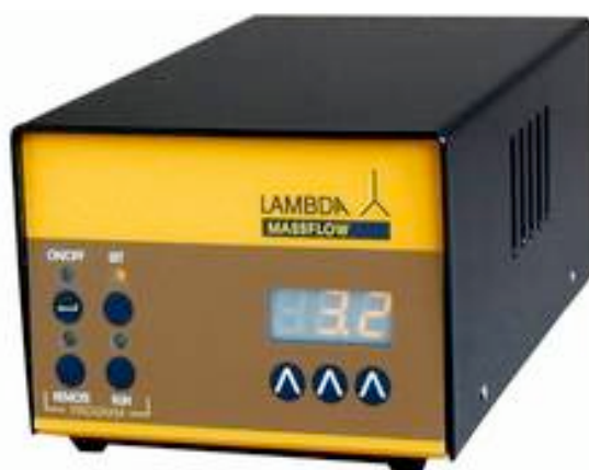
Figure 7: The lambda mass flow controller regulates cellular pO 2 and pH by monitoring the flow of oxygen and carbon dioxide through the culture. The system requires the purchase of additional electrodes to sense the O 2 and pH levels [8] .
