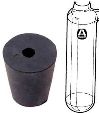
Figure 31: A rubber stopper like the one of the left enables the creation an air-tight seal when fitted into the cartridge. The hole in the center of the stopper will be used for the output tubing [19] . A glass cartridge like the one of the right will be MR compatible and can be autoclaved. The rubber stopper will fit into the top hole. The side port will be used for the input tubing [20] .
