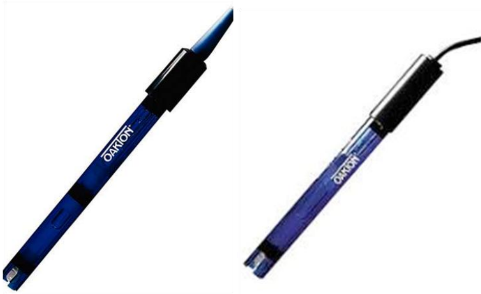
Figure 8: Oakton WD-E5642-50 DO probe [9] (left) and Oakton WD-35801-00 pH probe [10] (right). These electrodes sense DO and pH, respectively, and must be interfaced with a digital output source to convert data to relevant values.
