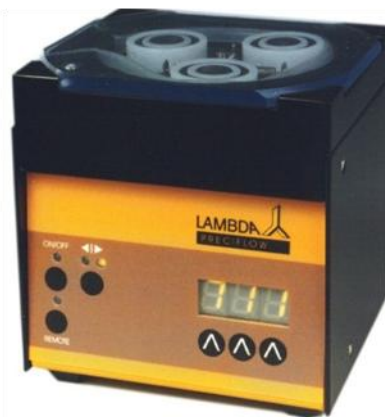
Figure 11: Peristaltic pump with glass bead bearings to compress the tubing and direct flow by the same means as a standard peristaltic pump, but with a reduced pulsation effect [13] .
