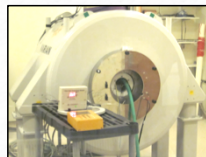
Figure 2: Micro MR Scanner. This scanner has a magnetic strength of 4.7 T. Items are placed in the central horizontal bore for scanning.
