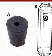
Figure 14: Examples of a Rubber Stopper (A) 16 and Glass Cartridge (B) 17 . A: Rubber enables the stopper to create an air-tight seal when fitted into the cartridge. The hole in the center of the stopper will be used for the output tubing. B: Glass is MR compatible and can be autoclaved. The rubber stopper will fit into the top hole. The side port will be used for the input tubing.
