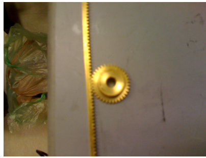
Figure 6: Rack and pinion to convert rotational motion to transverse motion.
