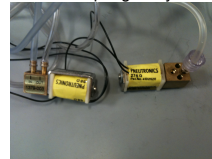
Valves: The left allows air into pressure compartment. The right lets air out.
