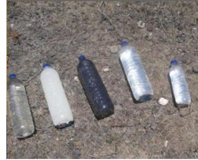
Figure 5: Example of water bottles coated with TiO 2 .
