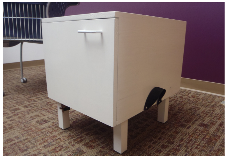
Figure 8: Completed box with side door. Final outer dimensions are 20"x16"x14.5"
