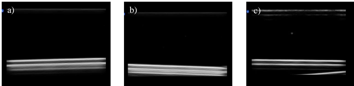
Figure 3 - Approximately 50mL of D5W (a), poloxamer solution (b), and poloxamer gel(c) was subjected to an Ultrasound System (SonixTOUCH). All of the images are quite clear, which will not inhibit ultrasound imaging during the ablation procedure.
